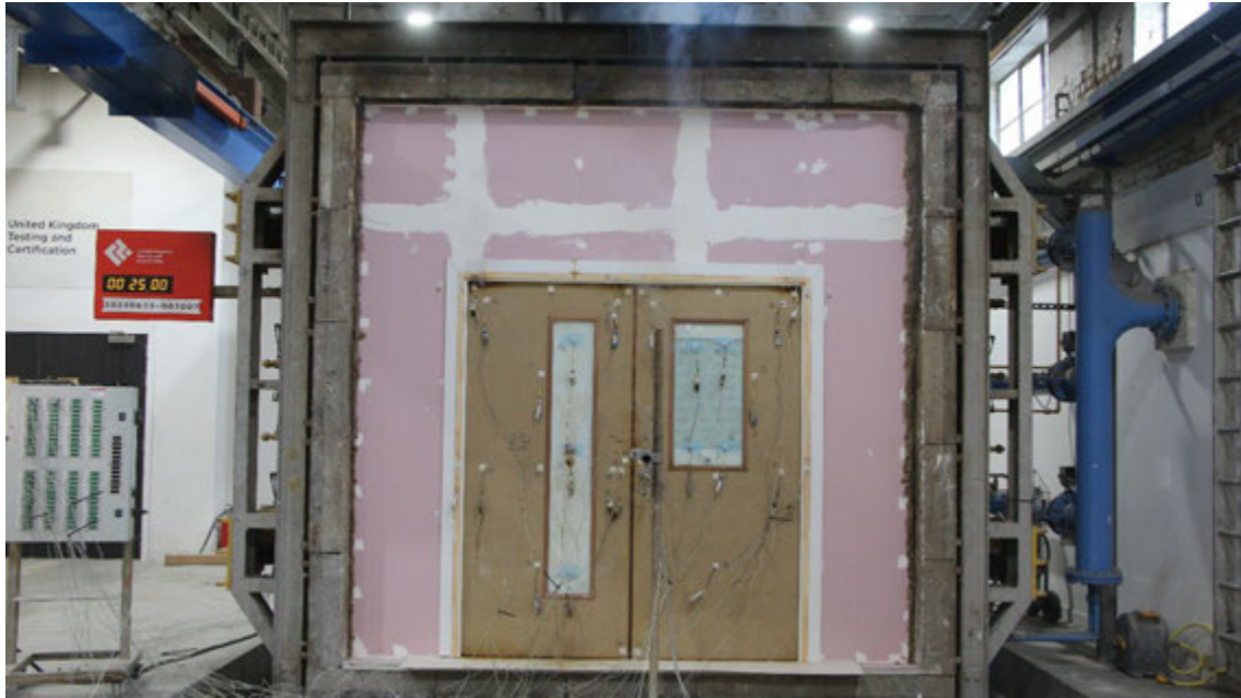
Figure 20 - The unexposed surface of the test construction after a test duration of 25 minutes
