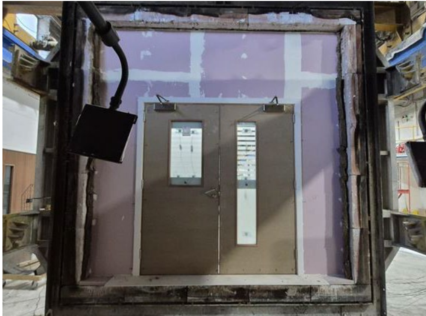
Figure 16 – The exposed surface of the test construction prior to commencement of the test
